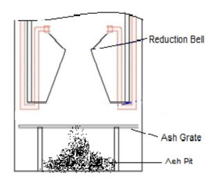
Figure 1: Schematic of Lower Part Reactor
