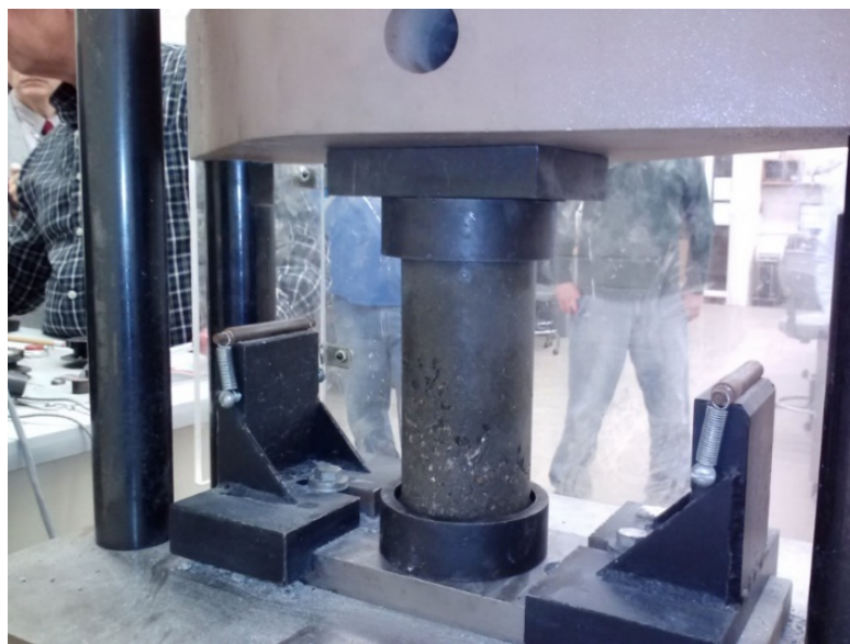
Figure 6: Typical sample loading in a universal testing machine.
