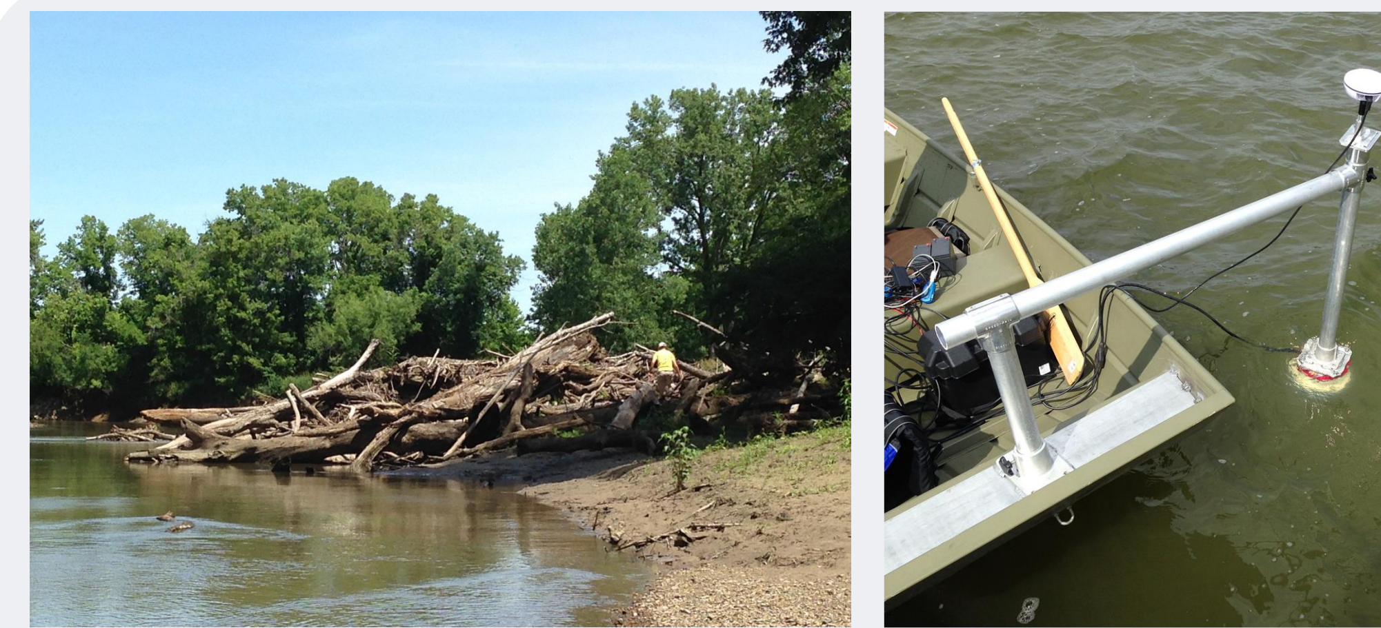
Figure 2 (left). Photograph of a portion of the LWD accumulation taken downstream on the main channel during summer 2014. Note the person for scale. Figure 3 (right). Data collection equipment mounted to the jon boat, including ADCP and differential GPS antenna.
