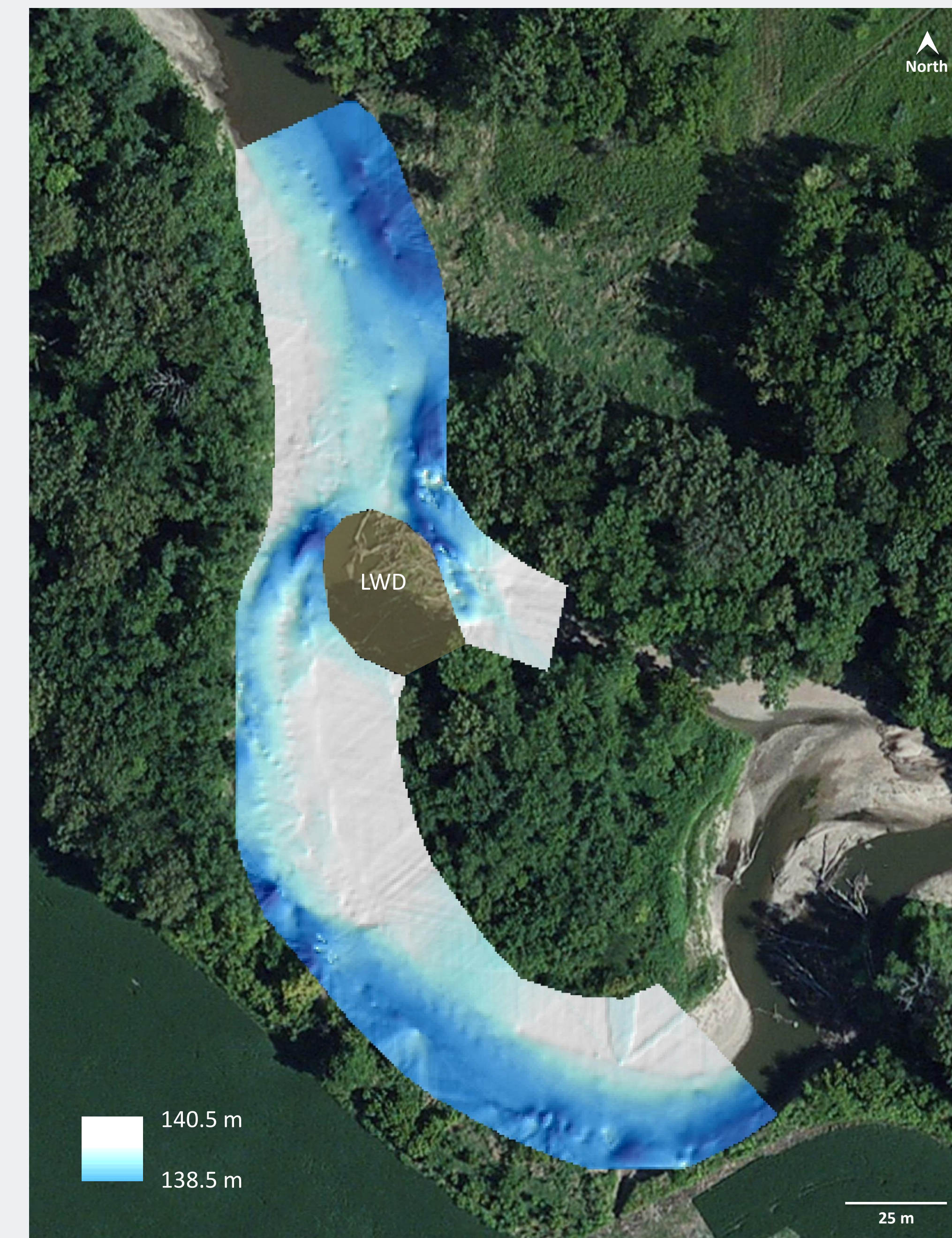
Figure 5. Bed topography of portions of the meander loop and chute cutoff, March 19, 2015. Elevation above sea level in meters.
